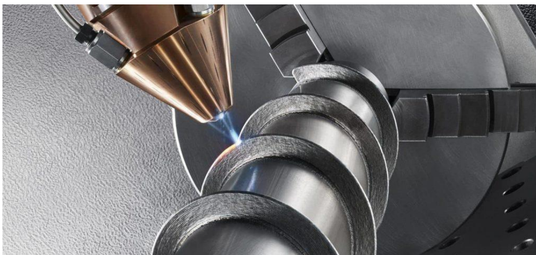
Obrázek 2-14: Metoda Directed Energy Deposition [40]
