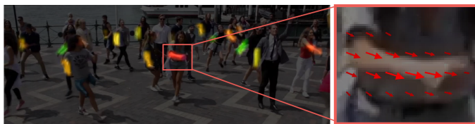
Figure 11: Left: Part Affinity Fields (PAFs). The color encodes orientation. Right: Illustration of vector field [3].
