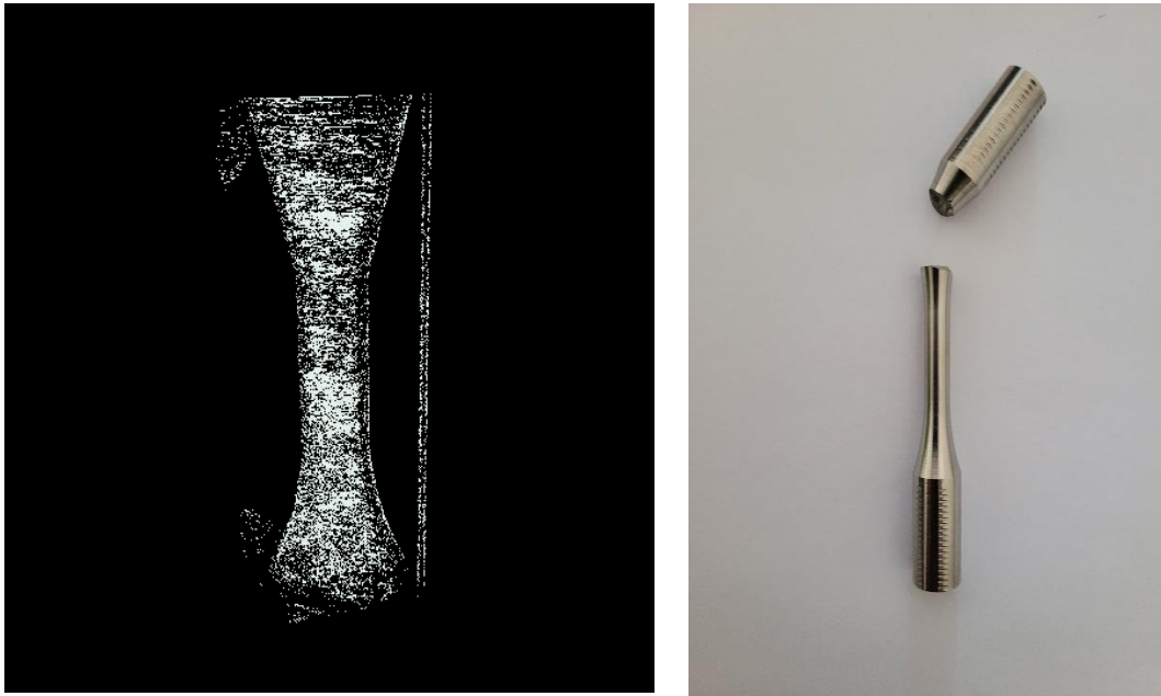
Figure 66 Another example for 3D view of high intensity(hot) spots of a part built with default settings and broken part after testing.
