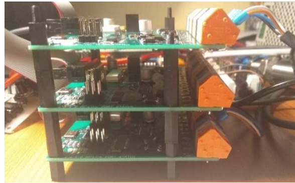
Fig. 8. Three IO-link master bridges with unique addresses in the sandwich.
