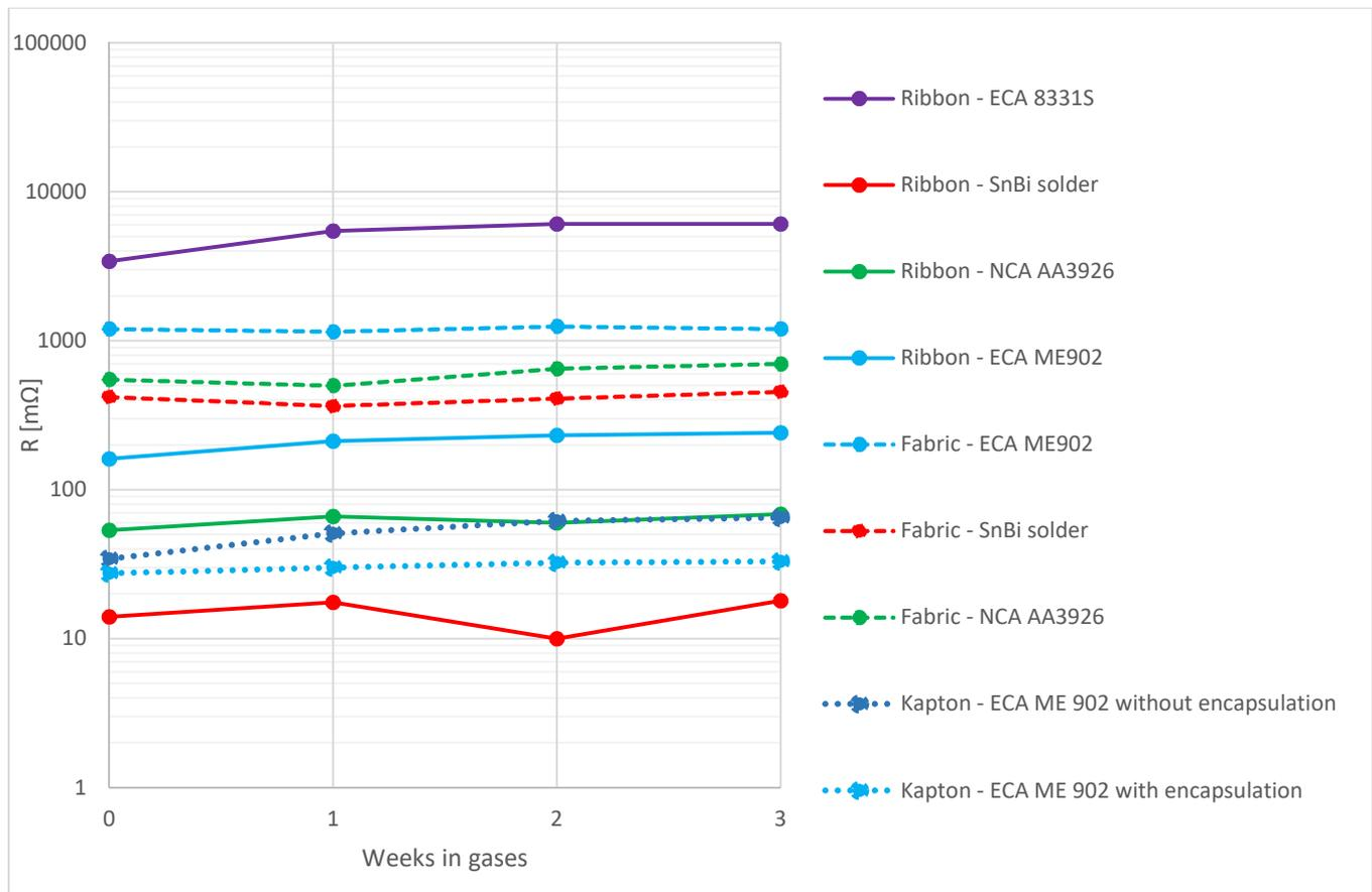
Fig. 5. Medians of electrical resistance for all samples.
