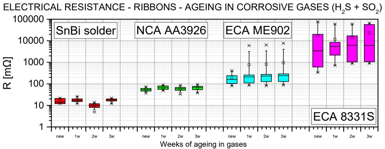
Fig. 2. The electrical resistance of ribbon samples – boxplot diagram.
