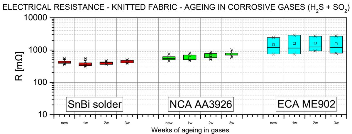
Fig. 3. The electrical resistance of knitted fabric samples – boxplot diagram.
