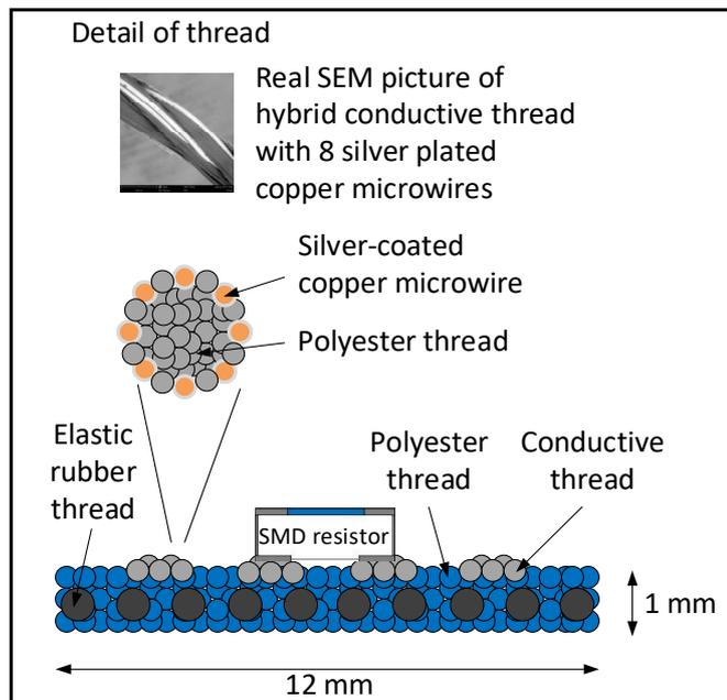
Fig. 1. Schematic cross-section of electrically conductive textile stretchable ribbons.
