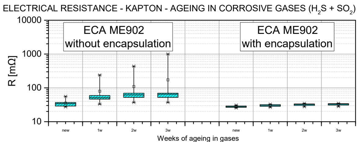
Fig. 4. The electrical resistance of kapton samples – boxplot diagram.
