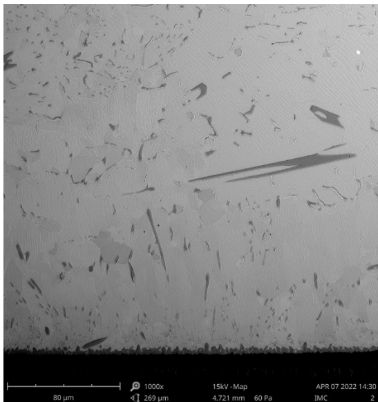
Fig. 10. Solder structure preview of SnNiCuGe
