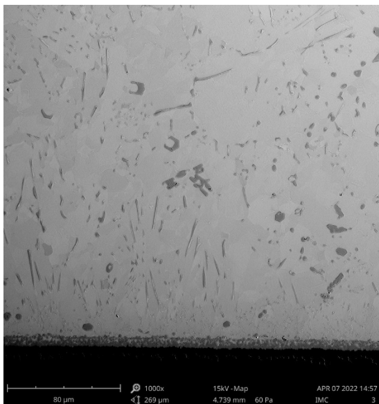
Fig. 11. Solder structure preview of SnNiCuCo
