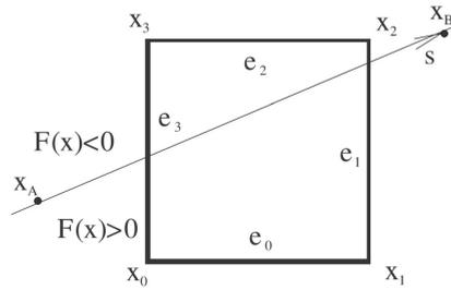
Fig. 5. Clipping against the rectangular window in  $E^2$ .
