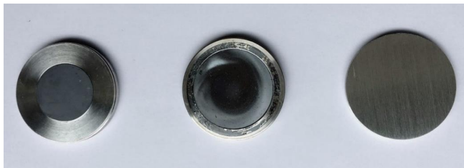
Figure 4-5: Composed Mg-Si targets with two various diameters (25 mm and 38 mm) and pure Mg target with a diameter of 50 mm.
