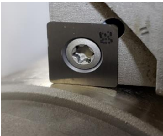
Fig. 1. Position of the cutting edge relative to the workpiece
