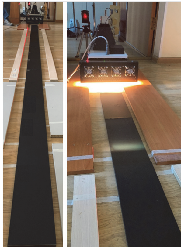
Figure 3: Inspection procedure using the LST device.
