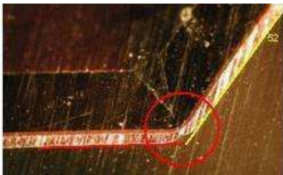
Fig. 1: Fig. 4 Cu cracks at the edge (bending angle 52^\circ )
