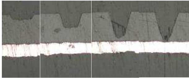
Fig. 3 Cross section of 'V' cut creation step-by-step
