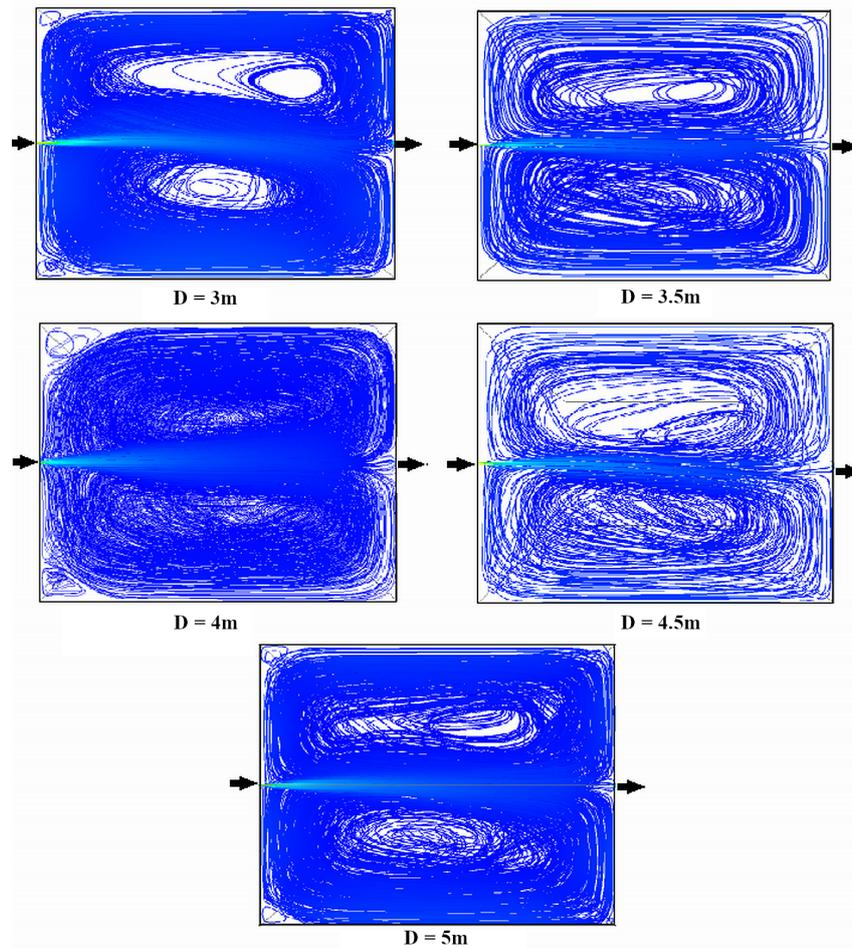
Fig. 8. Streamlines depicted in irrigation basins of different depths
