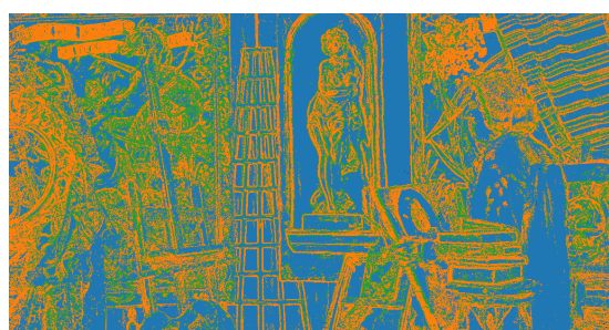
(c) Visualization of the classified regions. Blue: Lambertian; Orange: non-Lambertian; Green: outlier
