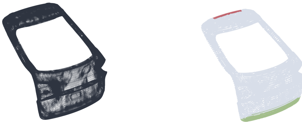
Fig. 2. The ground structure (left) and the boundary conditions (right). The clamped boundary conditions are the red nodes, the nodes with external forces are green
