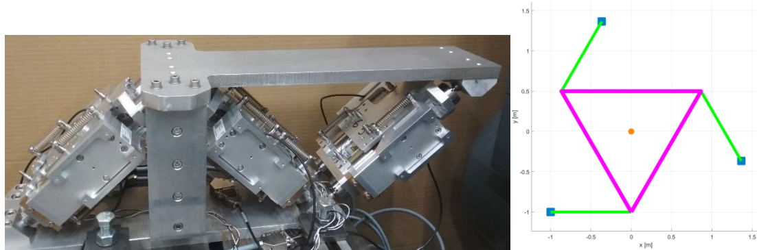
a) Perpendicular design of 3-DoF absorber b) Symmetrical design of 3-DoF absorber Fig. 1. Planar absorber kinematical configurations
