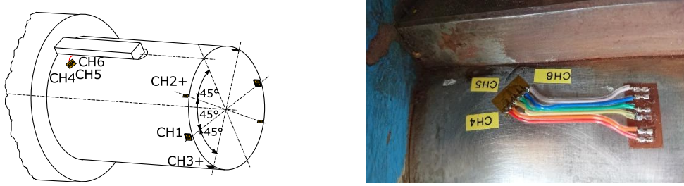
Fig. 2. The scheme of the location of the installed strain gauges (left) and detail of the strain gauge rose at the crack tip (right)
