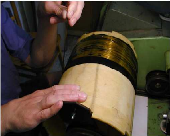
Fig. 11: Superconducting wire coiling
