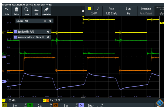
Obr. 12.35 Měření DAB, \phi_1 = 23 \text{ deg} , Pin = 609,6W, Vdc 48 V, Idc 12,7 A, Vout 53,4 V, Iout 10,4 A, Ch1 = TIM1 Ch1, Ch2 = TIM1 Ch1N, Ch3 = TIM1 Ch3, Ch4 = Itrafa
