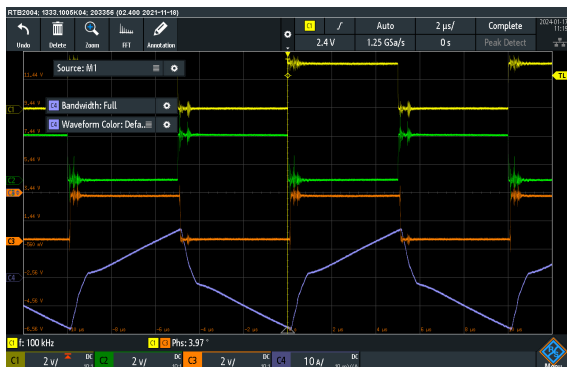
Obr. 12.28 Provoz DAB, V_{dc} = 48\text{ V} , I_{dc} = 8\text{ A} , \phi_i = 4\text{ deg} , V_{out} = 37\text{ V} , I_{out} = 7,5\text{ A} , Ch1 = TIM1 Ch1, Ch2 = TIM1 Ch1N, Ch3 = TIM1 Ch3, Ch4 = Itrafa
