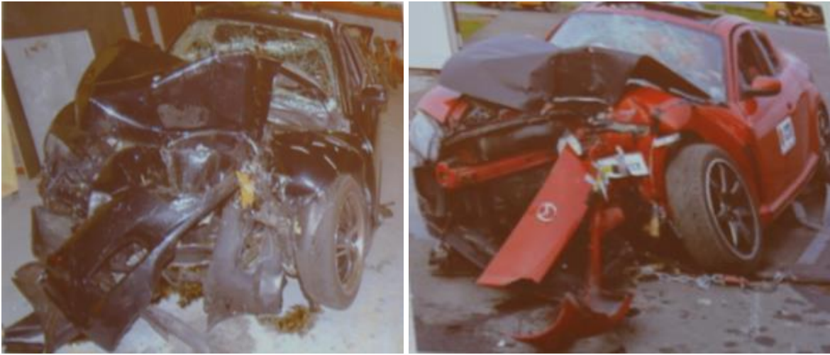
Figure 5.4 Vehicle after an accident vs. Vehicle after dedicated experimental reconstruction [119].
