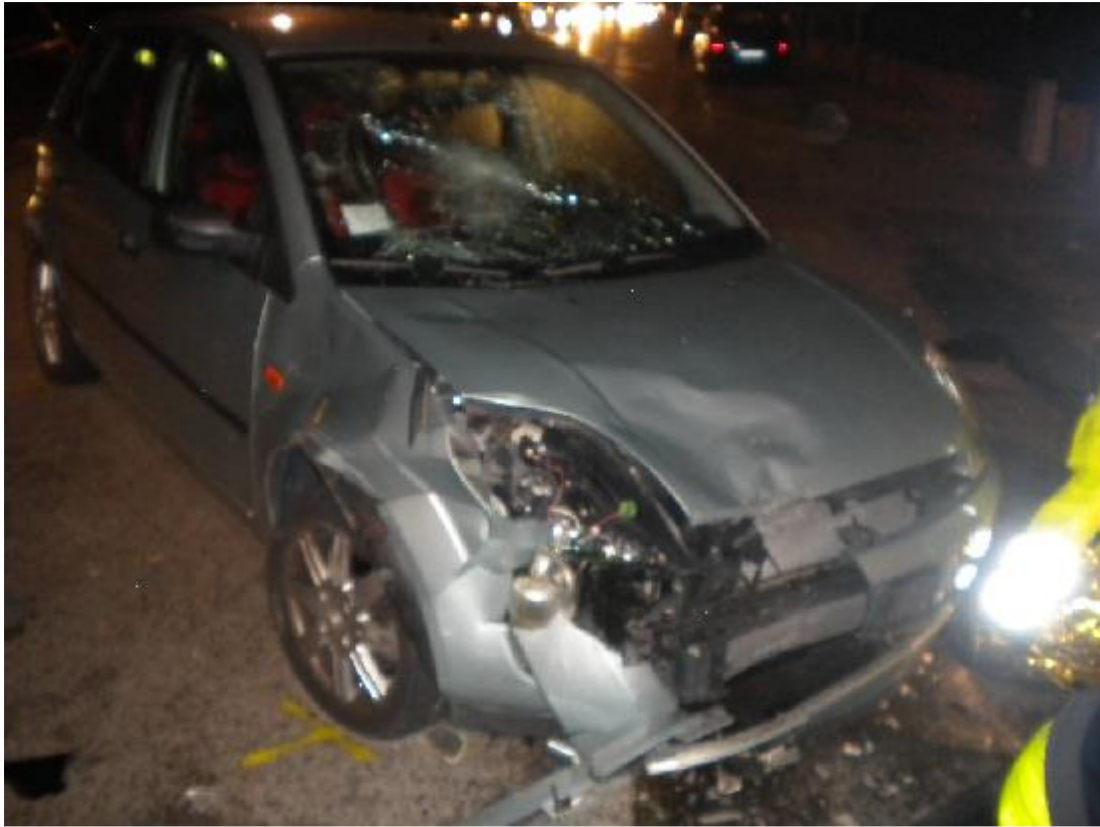
Figure 5.19 Case 1: Vehicle A crumple zone [154].
