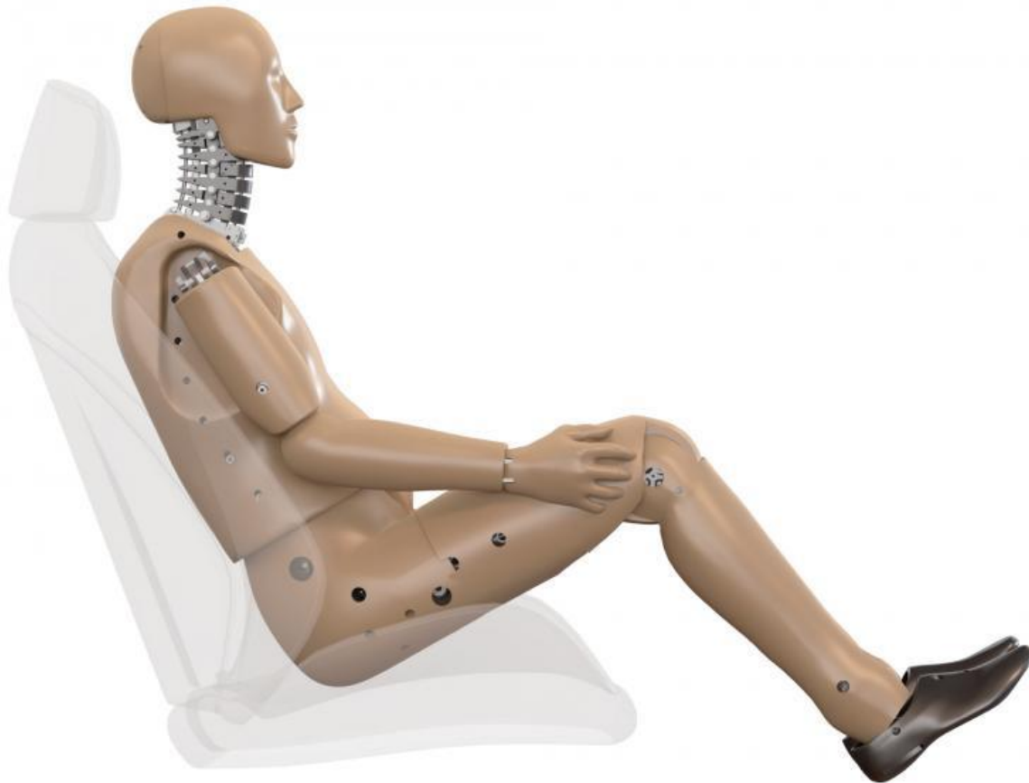
Figure 3.21 Side view of BioRID-II with the state-of-the-art neck for the rear impact scenarios purposes [36].
