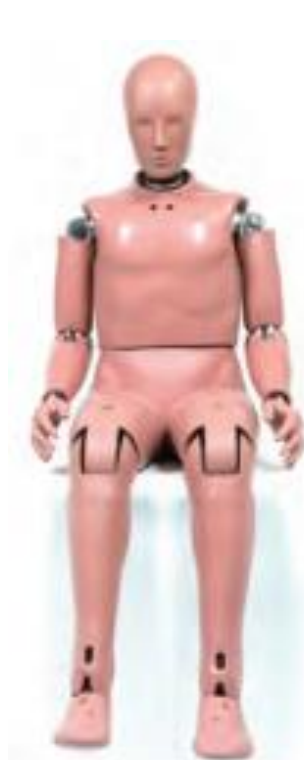
Figure 3.8 Hybrid III ATD [21].
