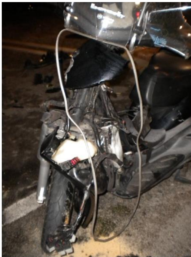
Figure 5.23 Case 1: Vehicle B bended front fork [154].
