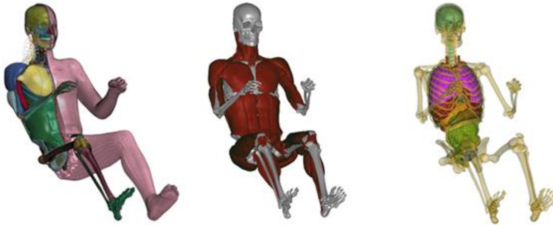
Figure 3.36 The GHBM base model (left - organs, middle - muscles and skeletal system, right - soft organs and skeleton).
