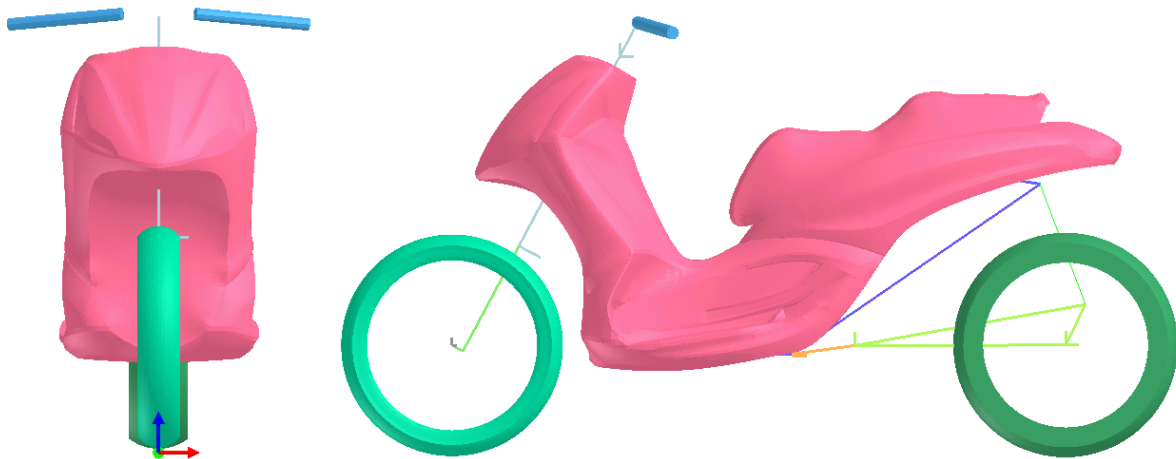
Figure 5.11 Implemented MBS model of maxi-scooter.
