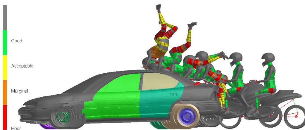
Figure 5.91 LMU case numerical reconstruction accident kinematics with the ongoing fast IC evaluation.
