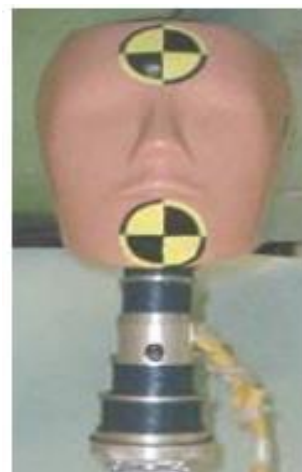
Figure 3.12 MATD head with the neck - frontal view [25].
