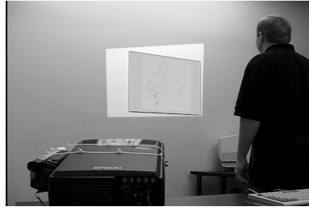
Figure 1: General monitoring and correction setup. (a) A framebuffer f is projected to a planar surface from a projector ( 2 in figure). A camera ( 1 in figure) observes the distortion and computes a framebuffer warp \hat{f} that simulates a projector at position 3 , whose optic axis is parallel to the display surface normal. Subsequent images are then monitored from 1 . (b) Depiction of an experimental setup. Camera-projector rig (in foreground) and corrected display. Although the intersection of the projected frustum with the display surface forms is not rectangular (illuminated quadrilateral), the framebuffer has been correctly pre-warped and the displayed image is geometrically correct.
