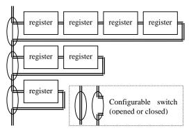
Figure 5. Configurable shift register.
