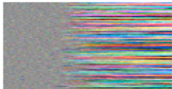
Figure 2: Color-mapped dimension representation of the atomic displacements relative to the perfect crystalline positions calculated over 3000 time steps (every 10 steps are skipped) across the solid-to-liquid phase transition in a 64-atom MgO system.
