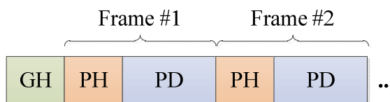
Fig. 1: LibPCAP file structure and frame layout
