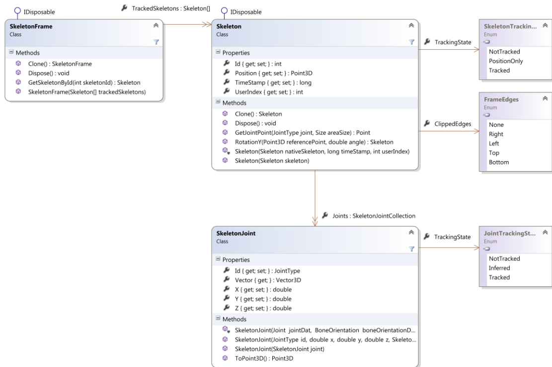
Figure 3.20 – A class diagram describing architecture of the skeleton frame data structure.
