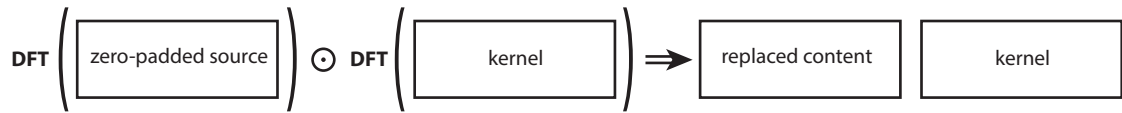
Figure 1.5: Transformation of the source and the kernel into new data that replace the source
