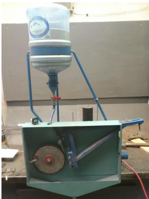
Obr. 37: Metoda Dry Sand/Rubber Wheel test
